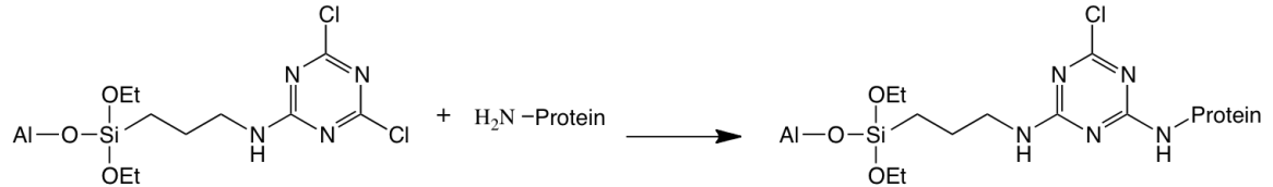
Figure 7: Schematic of the hTM protein reaction that couples to the TCT layer on a stent or flow diverter device.
