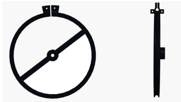
Figure 69: A multifunctional wheel designed in PTC Creo® to hold a Modified Chandler Loop, close it, and connect it to a motor shaft. The interior hole is designed to fit the motor shaft, while the flange on top provides both radial and longitudinal compression to close the tubing ends.
